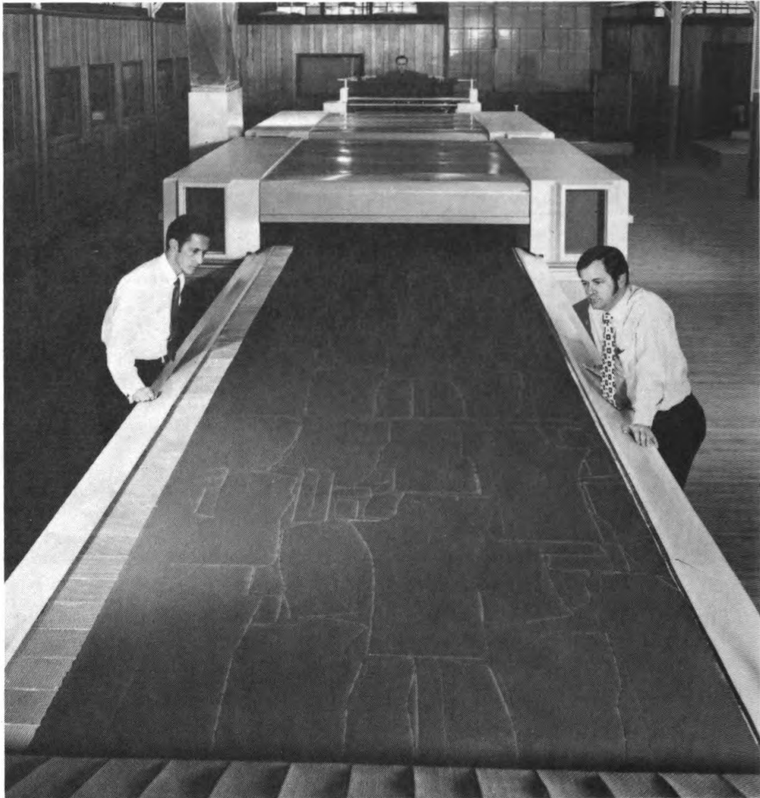
Figure 4. Engineers observe the results of cloth cutting performed by a computer-driven laser cutter.
